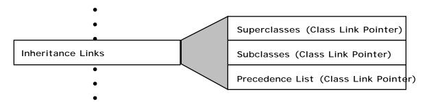
The inheritance links are lists of the direct superclasses, direct subclasses and inheritance precedence list of a class. All three of these lists are formed using an intermediary data structure called a **class link**. These lists are not formed using direct
