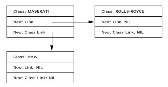
While an instance-set query function is executing, it uses a **Query Core** data structure to hold information about the query and instance-sets which satisfy the query. The data structure is summarized in the following diagram:
