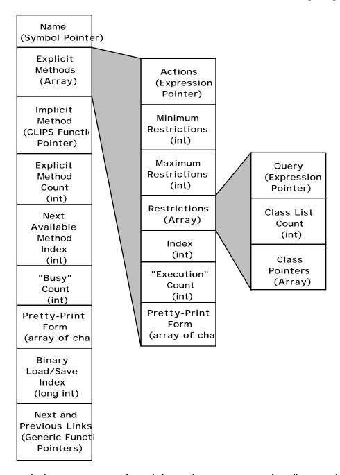
The internal data structure of a defgeneric construct primarily consists of: a symbolic name, an array of defmethod constructs (the explicit methods), a pointer to a
