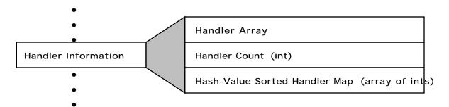
The message-handler information for a class is comprised of: an array of handlers, the number of handlers and an array of integer indices into the handler array which gives the order of the handlers according to the hash value of their symbolic names. The sorted handler map allows a handler to be found easily by performing a binary search on the symbolic hash value of the handler name. For details on the message-handler data structure, see the Message-Handler Commands Module.
