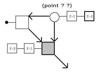
The process of updating the bottom join for the addition of f-2 is complete. Notice that the beta memory of the top join never contains any partial matches. Joins that correspond to the first pattern of a rule will never make use of the beta memory.
