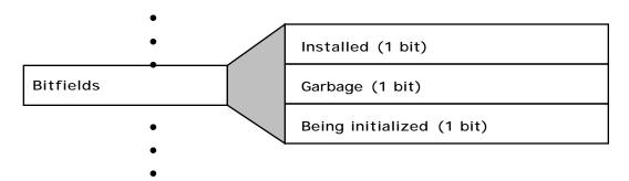
The bitfields are stored in a single integer and indicate the following information about an instance: whether all the atoms within the instance have had their busy counts incremented (i.e. whether the instance has been installed), whether the instance has been functionally deleted (i.e. the instance on the garbage list) and whether the instance is in the process of being initialized by **make-instance** or **initialize-instance**.
