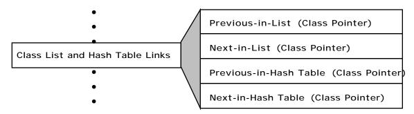
Unlike the inheritance links, the links which place a class in the global class list (ClassList) and class hash table (ClassTable) are implemented with direct class pointers in the defclass. This is because these links are unique to a class.
